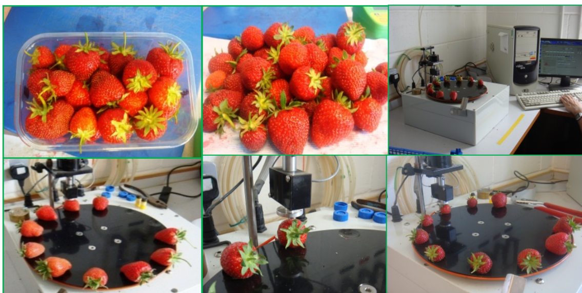
Figure 1. Harvested strawberry fruits and measuring fruit firmness using Firmtech.
